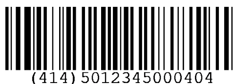
Figure 12: An example of a GLN for a physical location encoded to a GS1-128 barcode
