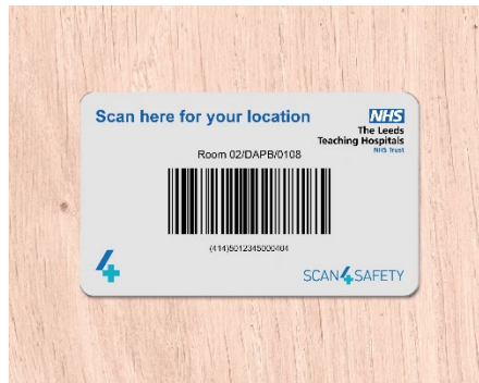
Figure 13: An example of a GLN for a physical location encoded to a GS1-128 barcode in practice
