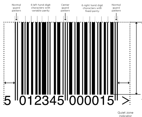
Figure 29: General format of an EAN-13 barcode
